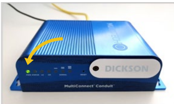
Figure 7 – Power indicator remains on when gateway is ready to use
