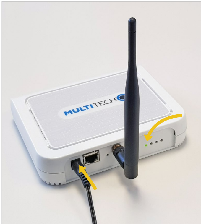
Figure 8 – Plug in the power cable into the power plug
