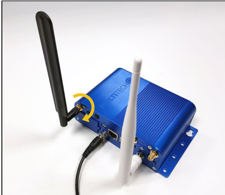
Figure 22 – Fasten the cellular radio antenna (on left)
