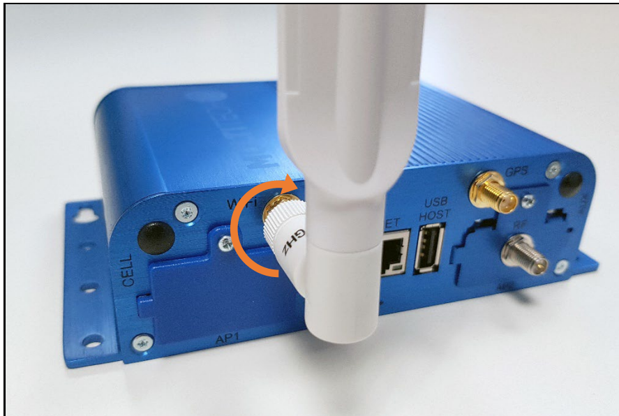
Figure 15 – Attaching antenna for Wi-Fi network
