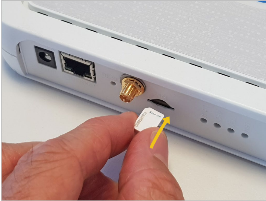
Figure 24 – Insert SIM card completely into slot
