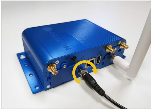
Figure 6 – Plug in the power cable to the stainless-steel connector
