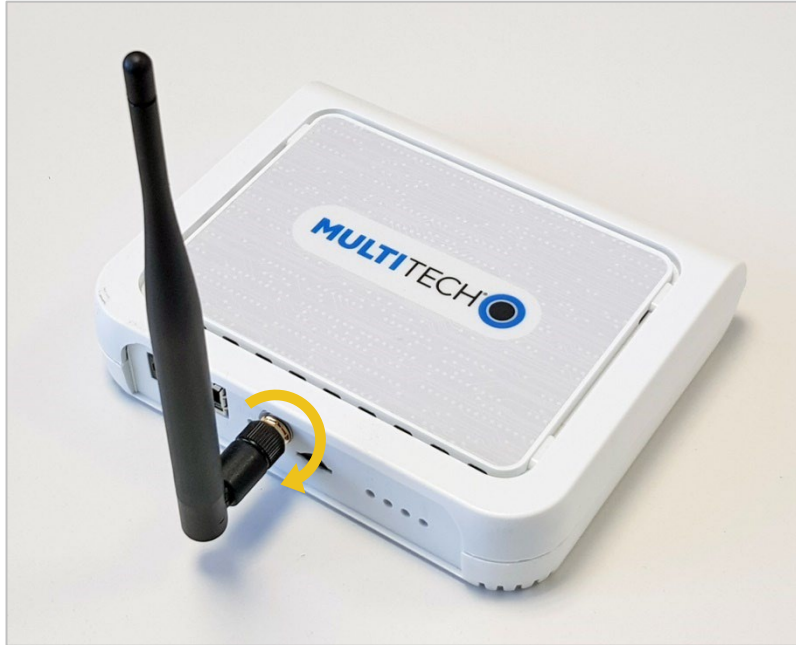
Figure 5 – Attach LoRaWAN antenna to the connector
