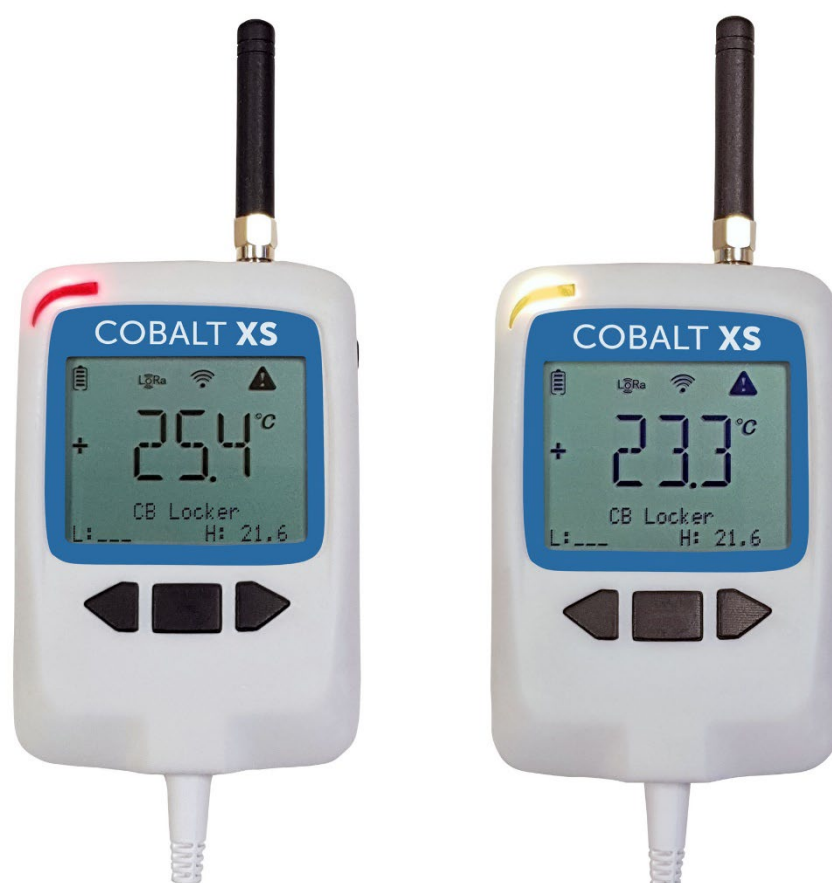
Figure 16 – Data logger with alarm (left) and warning (right)
