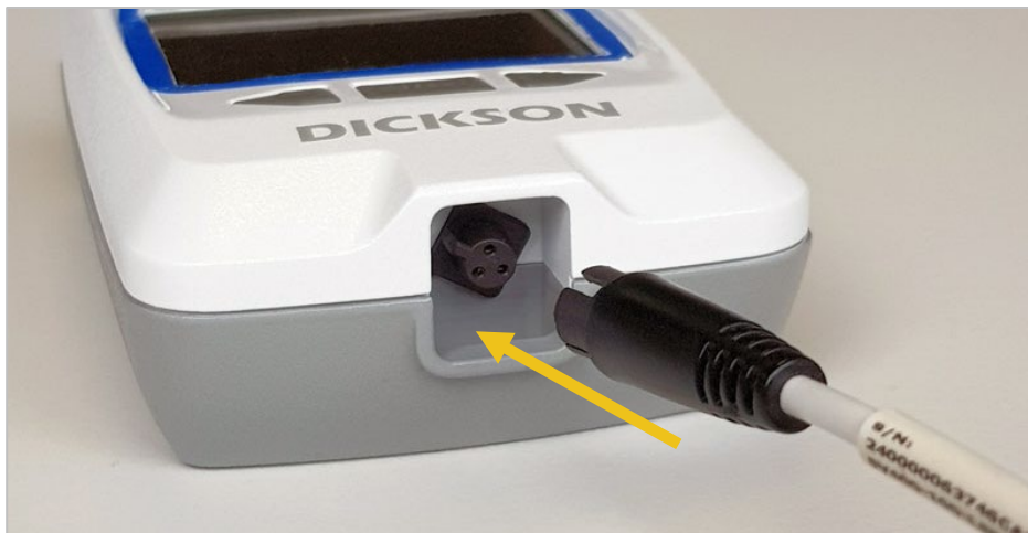
Figure 12 – Plugging a sensor into the Cobalt XS data logger
