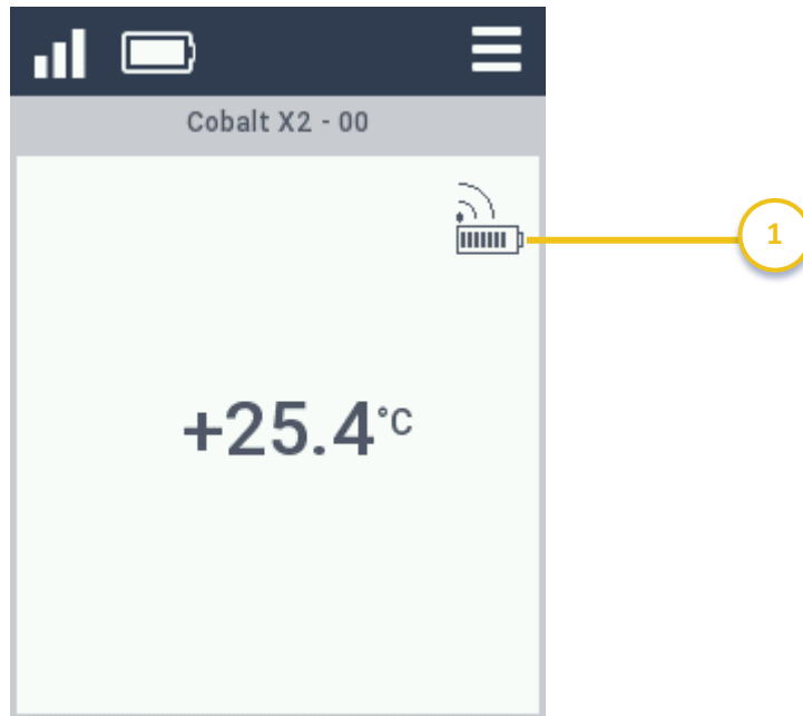
Figure 65 – Display showing one of the sensors as a remote (wireless) sensor
