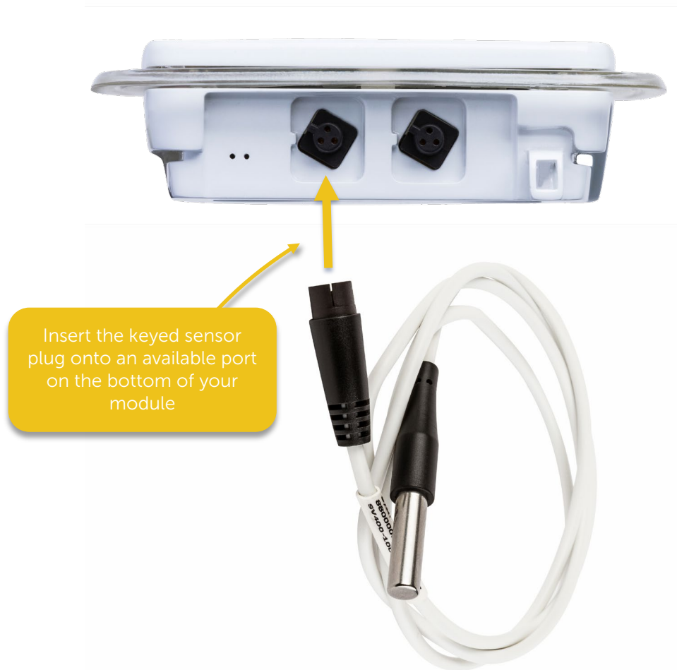
Figure 22 – Cobalt X data logger with external digital sensor
