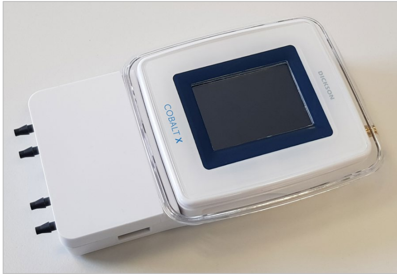
Figure 43 – Slide the Smart-Sensor extension onto the Cobalt X data logger
