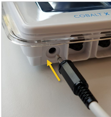
Figure 45 – Insert jack into dry contact input plug
