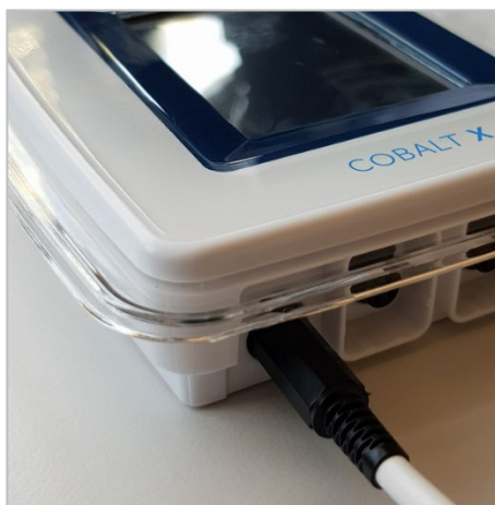
Figure 46 – Cable inserted into input jack on data logger
