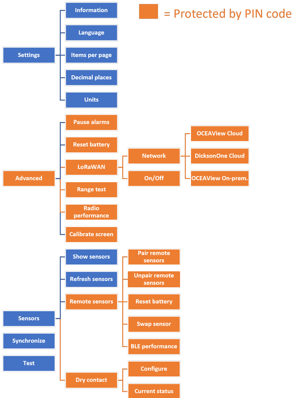
Figure 69 – Menu structure when using LoRaWAN wireless operation
