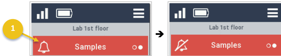
Figure 99 – Bell icon indicating that alarm sound is active
