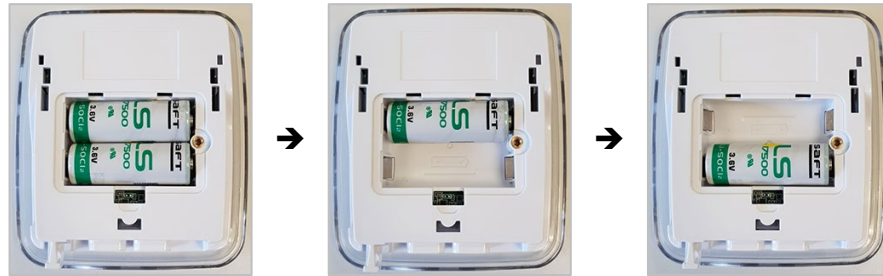
Figure 108 – Replace one battery after the other (and/or keep AC power on)
