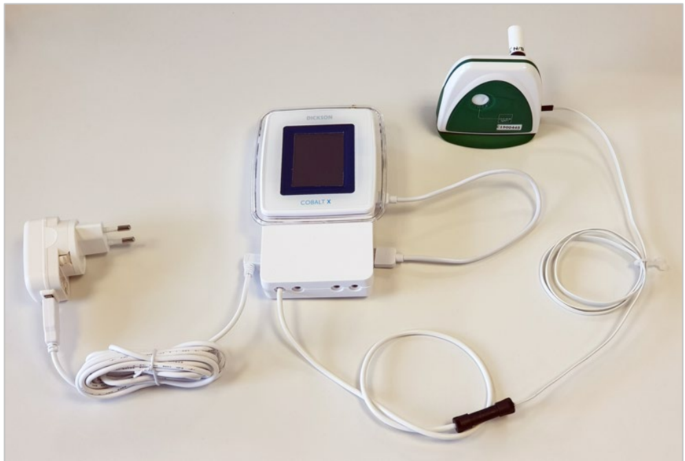
Figure 34 – Fully connected triple sensor assembly
