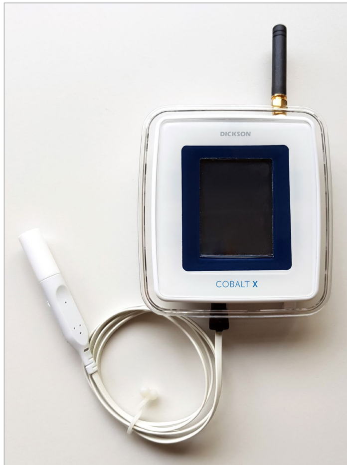
Figure 25 – Cobalt X data logger with dual temperature-humidity sensor
