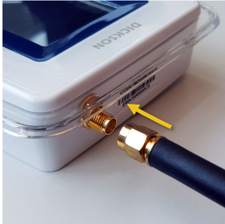
Figure 11 – Place antenna on connector
