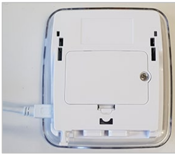
Figure 106 – Optional: plug in USB power to avoid losing data
