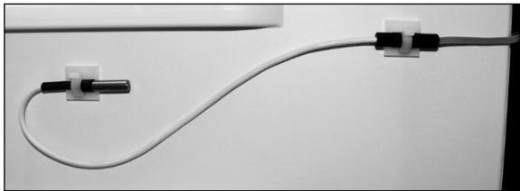
Figure 23 – Sensor inside refrigerator chamber (external sensors only)
