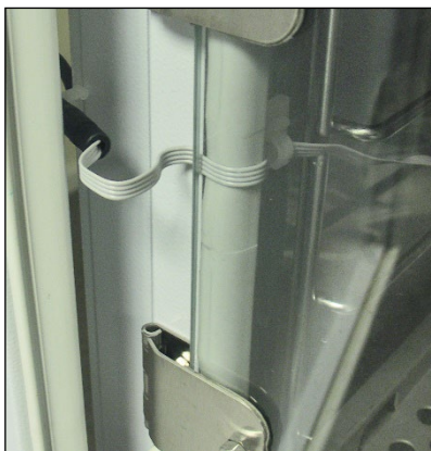
Figure 28 – Ribbon cable lays flat beneath door joint
