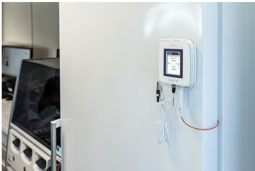
Figure 24 – Cobalt X data logger mounted on the refrigerator door
