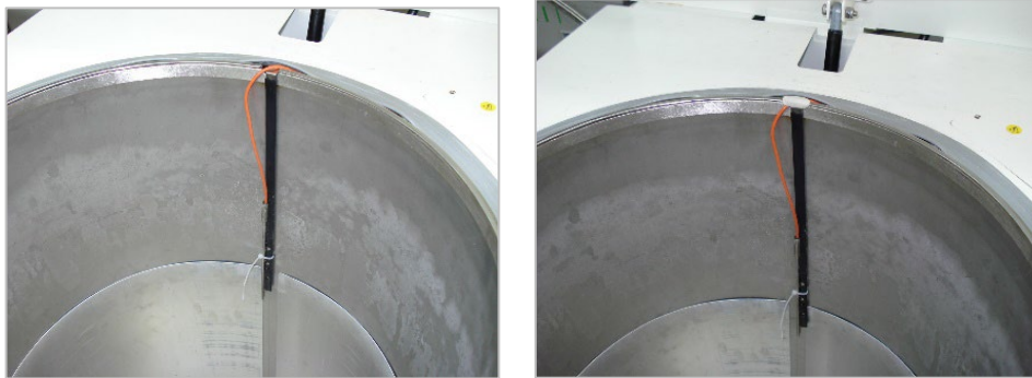
Figure 20 – Pt100 (-200°C to +50°C) for nitrogen/cryogenic tank
