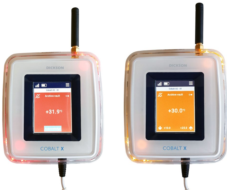
Figure 97 – Data logger with alarm (left) and warning (right)
