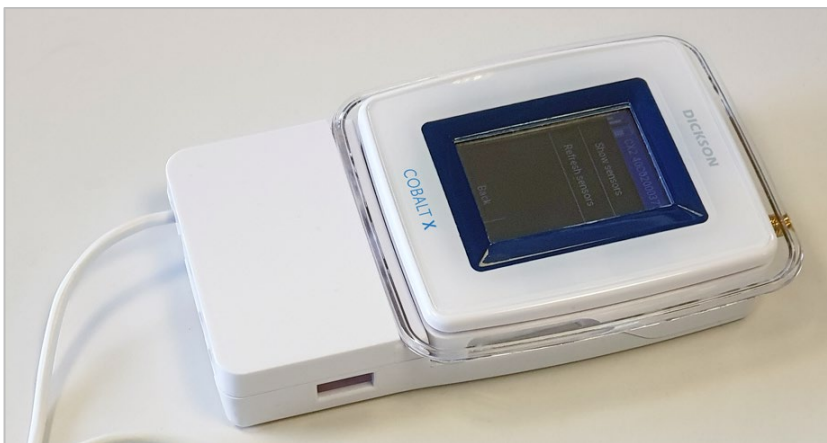
Figure 30 – Slide the Smart-Sensor extension onto the Cobalt X data logger
